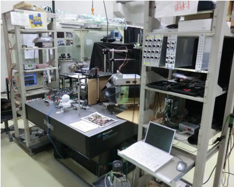
Fig. 7.12 The entire appearance of the apparatus. The vacuum enclosure on the turntable covered with black sheet is the main optical component, and the laser source is placed on top . Some electrical circuits and web camera are also put on the optical table. The rack on the left has the PZT driver and the data logger we used for the data acquisition. The rack on the right has the motor driver and the PC for controlling the motor for the turntable
